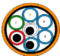
Sub divided Sub-duct
